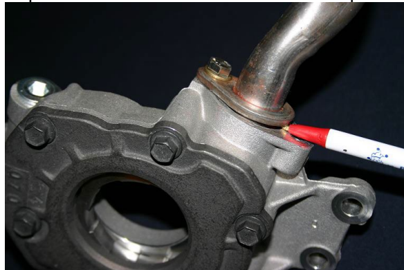
(This pickup tube is NOT installed correct)
