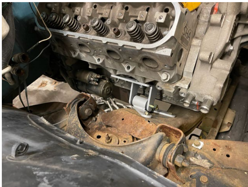
, (Detailed view of driver's side motor mount and frame bracket in chassis)
